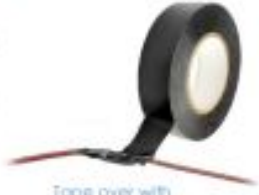
Tape over with insulating tape
